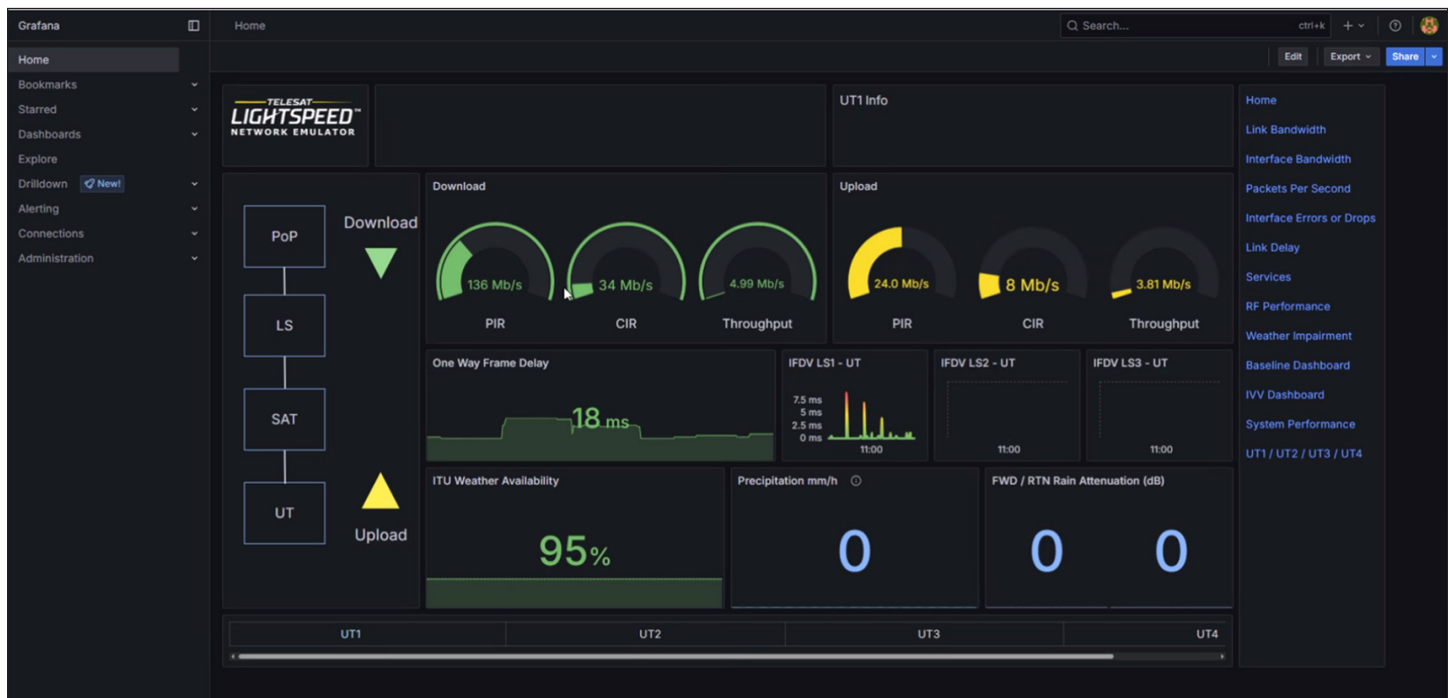
Figure 19. Telesat's LEO Emulator: LEO intra/inter Satellite Profile with live traffic
