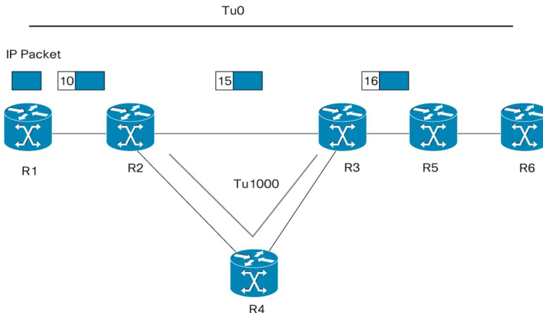
A primary LSP (Tunnel 0) is configured from R1 to R6 (Figure 8). The link between R2 and R3 via FRR should be protected. A backup “tunnel,” which will only be used when a failure occurs, is statically configured on R2 going to R3 across R4. When configuring this particular tunnel, the links used by the primary tunnel cannot be used.
