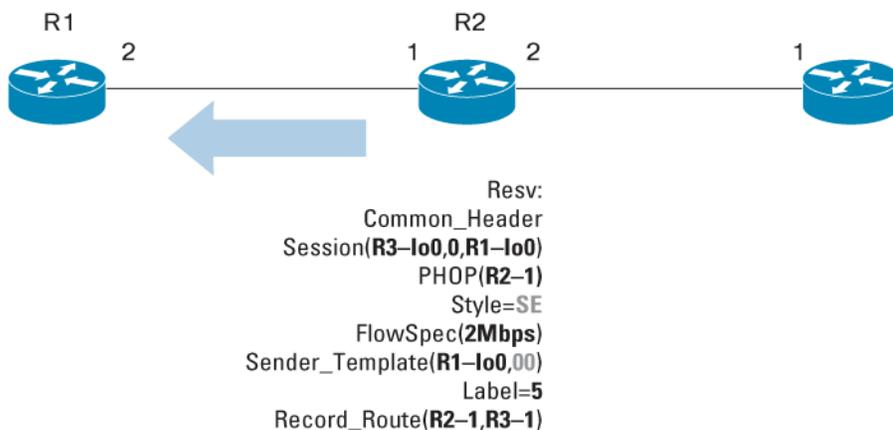
Step 8. LSP is established, any outgoing packets on R1-2 will be tagged with Label=5. Next step is to send the traffic down this LSP either by static route, Autoroute announce or Policy based Routing.
