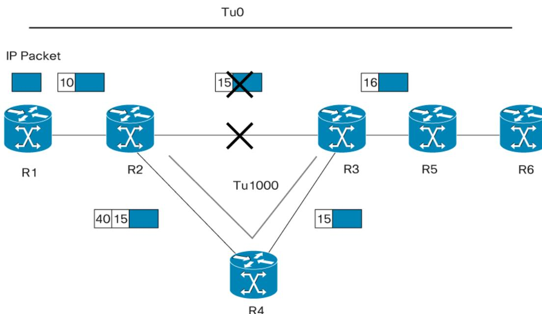
Upon link failure (Figure 9), R2 rewrites all the incoming labels to go over the backup link. As a result, R2 will reroute traffic around the failure by sending packets into a different downstream interface.
