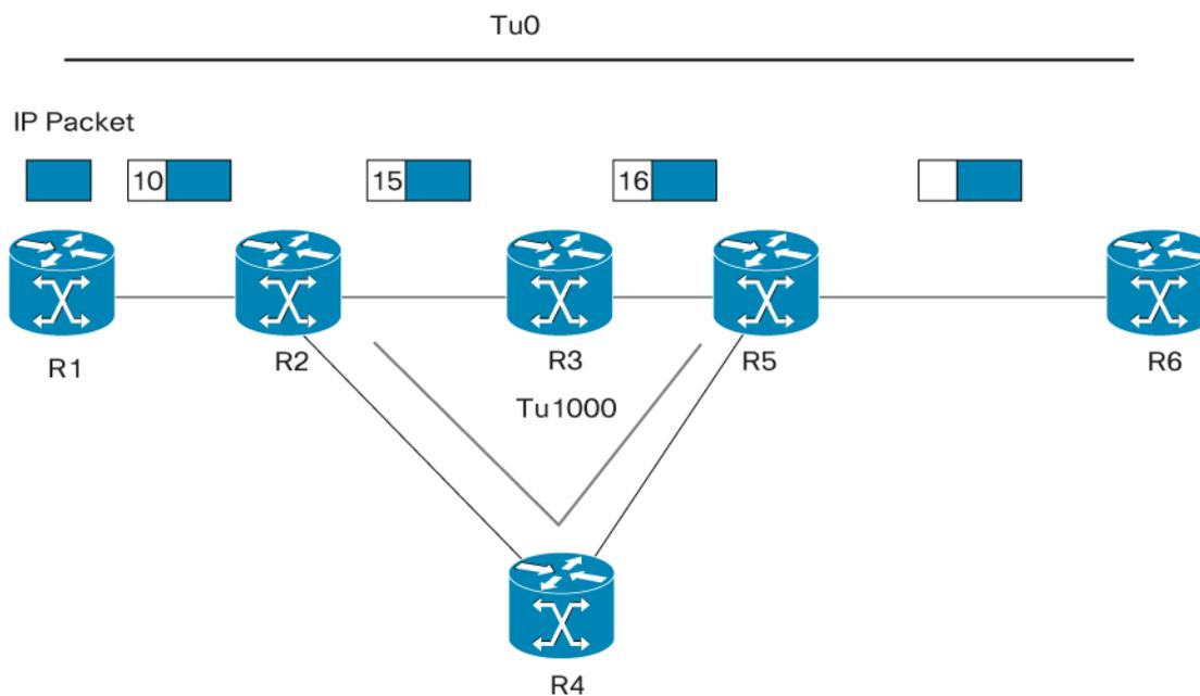
In this scenario (Figure 10), consider a primary LSP: R1-R2-R3-R5-R6. Protecting the node R3 is achieved either through a) R2-R4-R5-R3 or b) R2-R4-R5. In the case of a), the backup path being R1-R2-R4-R5-R3-R5-R6, this is the same as the backup tunnel to the next-hop. Notice though, that the (R3, R5) link will carry the traffic to R6 twice (i.e. double reservation). This solution is not optimal.
