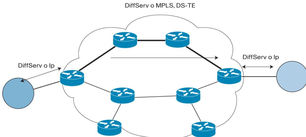
Consider the architecture defined in Figure B2. We would like to enforce DiffServ from end-to-end. The two IP clouds respectively on the left and right of the MPLS cloud are already DiffServ aware. The goal is to extend DiffServ support into the MPLS cloud.
