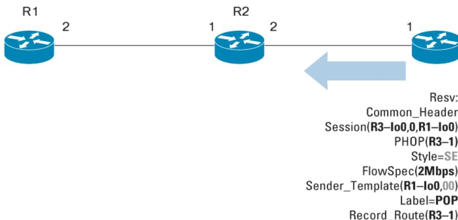
Step 6. R2 will forward any incoming packet from interface R2-1 to interface R2-2, at the same time R2 will POP the label for the outgoing packets.
