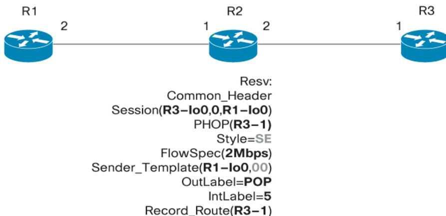
Step 7. RESV message R2-R1, R2 requests R1 to use label=5 for any packets on the link R1-2/R2-1 destined to R3
