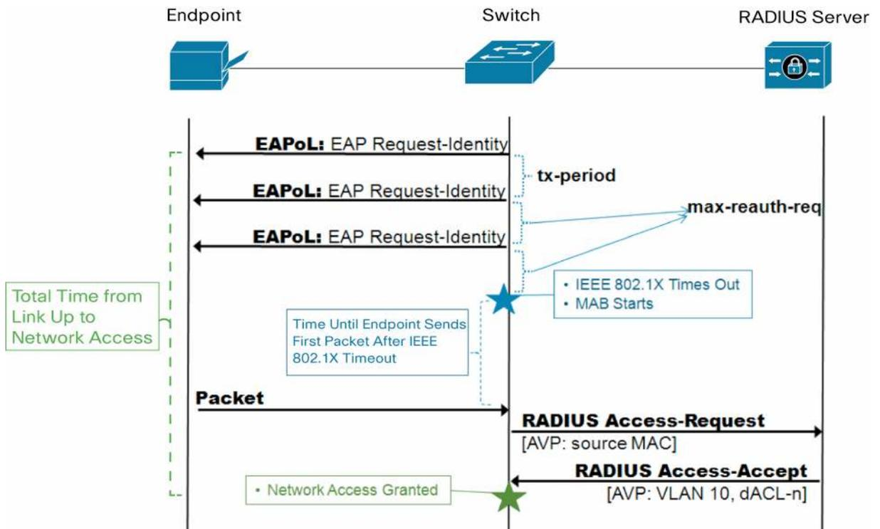
The combination of **tx-period** and **max-reauth-req** is especially important to MAB endpoints in an IEEE 802.1X-enabled environment. MAB endpoints must wait until IEEE 802.1X times out before attempting network access through a fallback mechanism. The total time it takes for IEEE 802.1X to time out is determined by the following formula:
