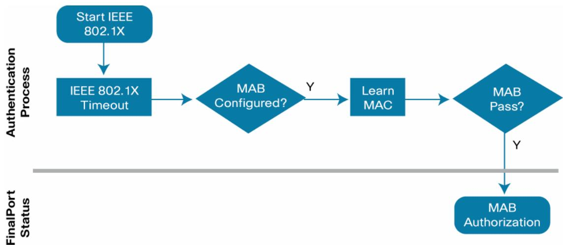
When configured as a fallback mechanisms, MAB is deployed after IEEE 802.1X times out. If the endpoint's Pre-Execution Environment (PXE) process times out, or if Dynamic Host Configuration Protocol (DHCP) gets deep into the exponential backoff process before the timeout occurs, the endpoint may not be able to communicate even though the port has been opened. To the end user, it will appear as if network access has been denied. There are three potential solutions to this problem:
