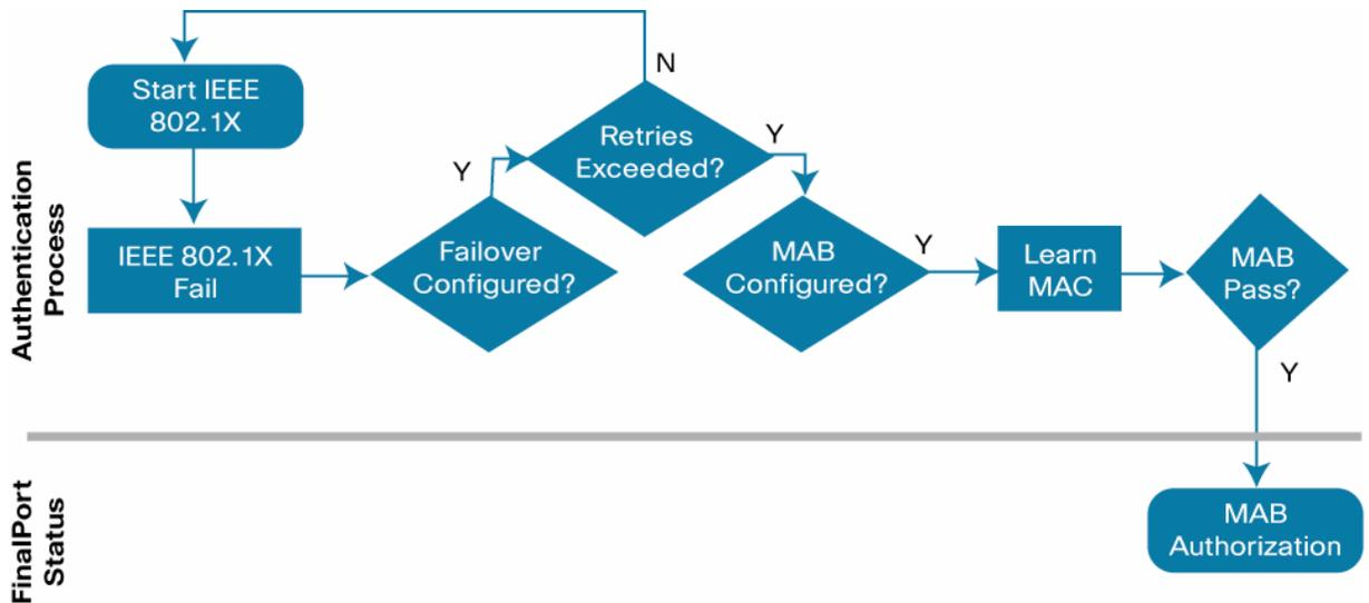
Because MAB begins immediately after an IEEE 802.1X failure, there are no timing issues. However, to trigger MAB, the endpoint must send a packet after the IEEE 802.1X failure. In other words, the IEEE 802.1X supplicant on the endpoint must fail open.
