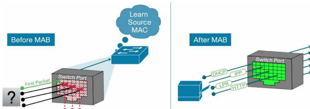
Prior to MAB, the endpoint's identity is unknown and all traffic is blocked. The switch examines a single packet to learn and authenticate the source MAC address. After MAB succeeds, the endpoint's identity is known and all traffic from that endpoint is allowed. The switch performs source MAC address filtering to help ensure that only the MAB-authenticated endpoint is allowed to send traffic.
