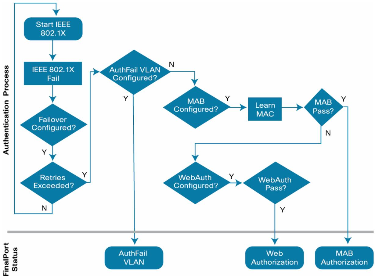
In this sense, AuthFail VLAN and MAB are mutually exclusive when IEEE 802.1X fails. However, you can configure the AuthFail VLAN for IEEE 802.1X failures (the client has a supplicant but presents an invalid credential as shown in Figure 9) and still retain MAB for IEEE 802.1X timeouts (the client has no supplicant as shown in Figures 7 and 8).
