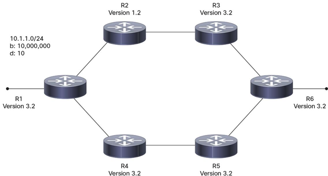
For the routers running the older versions, EIGRP will use the interface reporting the delay of 100 milliseconds, and the bandwidth value of 10,000,000 kilobytes/second.
