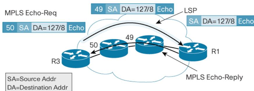
LSP traceroute is a data plane verification tool that traces LSP paths in the MPLS network. In the trace route LSP verification, the packet is sent to the control plane of each transit LSR, which performs various checks to ensure that it is indeed a transit LSR for this path.
