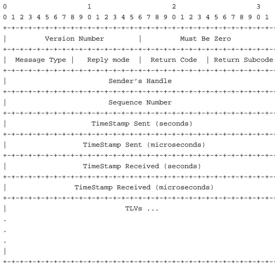
Message Type field identifies whether the UDP payload is an MPLS echo request or MPLS echo reply.
