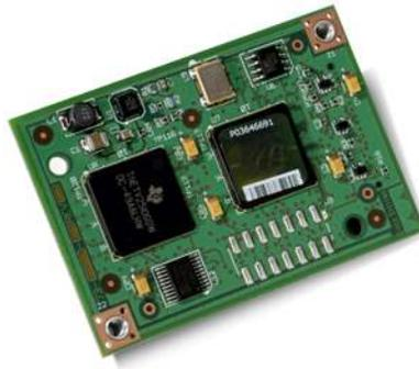
**Figure 2.** Cisco 2-Port T1/E1 MFT VWIC2 with 64-Channel MFT Dedicated ECAN Module
