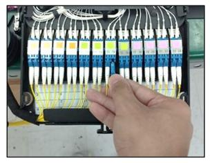
**6.5.3.7.** Route the cable underneath the cable protection flap to join it with the bundle. Make sure to not pinch any of the cables when doing so. Guide the cable towards the black plastic ring clip from the front cable sleeve. Insert the cable into the split sleeve.
