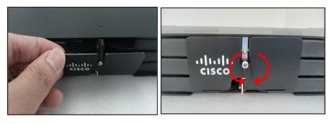
**5.2.1.9.** Put back the cable sleeve to the cable hanger arm
