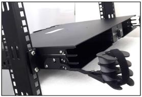
**4.2.3.** Open the front door of the chassis by turning the front door handle clockwise or counter clockwise to the open position, partially withdraw each cassette installed, open the front portion of each unit and remove and discard the protective foam.
