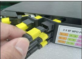
**4.3.1.2.** For MPO jumper cable connections on the rear door, please provide at least ten inches (10") cable slack as provision for rear door opening clearance.
