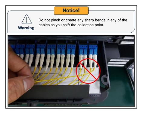
**5.2.1.3.** Guide the cable bundle towards the black plastic ring clip from the front cable sleeve. Be sure the bundle is beneath the cable protection sleeve so as not to pinch any of the cables when doing so. Insert the cables into the split sleeve.
