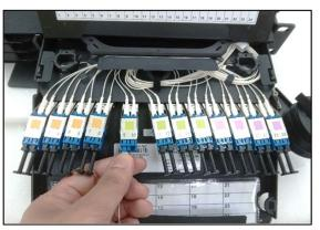
**5.1.9.** Repeat steps 5.1.5 through 5.1.8 for any additional connectors that need to be inserted into the front side of the adapters.
