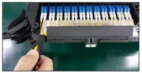
**5.2.1.4.** Pull the black plastic ring clip from the front cable sleeve to easily complete the cable insertion.
