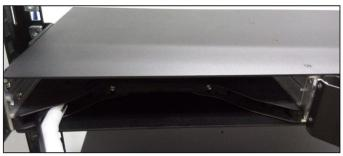
**4.3.2.5.** Get another cassette and insert the front cable sleeves (black) into the chassis (5a). position and push to insert the cassettes on the middle slot of the chassis (5b).
