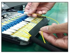
**6.5.3.6.** To insert the replacement jumper, push horizontally on the connector housing until it is fully seated in the adapter. An audible click will be heard when it is properly inserted.
