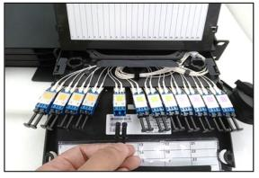
**5.1.8.** To insert the connector into the adapter, simply push horizontally on the housing of the connector until it is fully seated in the adapter. An audible click will be heard when it is properly inserted. (Reminder: Inspect, clean, Inspect, connect both sides of the connector (ICIC)).
