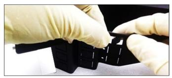
**4.3.2.3.** Install MPO adapters in each knockout of chassis. Ensure the correct orientation of the adapter is maintained.
