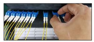
6.5.1.3. While gently depressing the connector latching tab, pull on the connector housing to un-mate the connector plug from the adapter.
