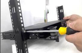
**4.2.2**. To straighten the cable hanger, move the head of the cable hanger by swinging it outwards the chassis until it locks into place.
