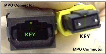
**4.3.2.9.** Insert MPO Connector(s) from the cassette into the MPO adapters on the back door. Push MPO connector in until a "click" sound is heard upon attachment. Ensure the right orientation of MPO Connector and MPO Adapter (e.g. KEY-UP)
