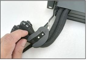
**6.3.2.** Slide out the cassette, press down on the front tab, and lift up the flap to expose the jumper cables.
