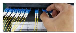
**6.5.2.3.** Lift the flap which covers the rear plane of the connector shelf; using one hand to support the bottom of the adapter, gently depress the connector latching tab to unlock and remove the connector from the adapter.
