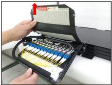
**6.3.3.** Separate a jumper by gently pulling it out of the black cable sleeve. When needed, remove other cables or the rest of the bundle from the cable sleeve as well.
