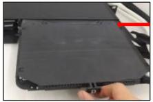
**5.1.4.** Press down on the front tab, then lift up the lid, loosen all the cassette snaps, and then the adapters will be exposed.
