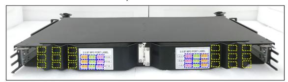
**4.3.2.2.** Open the rear door and remove all 3 knockouts associated with each cassette to be installed in the chassis. The number of knockouts should match the number of MPOs to be installed.
