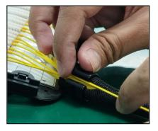
**6.5.3.8.** Pull the black plastic ring clip from the front cable sleeve to easily complete the cable insertion.
