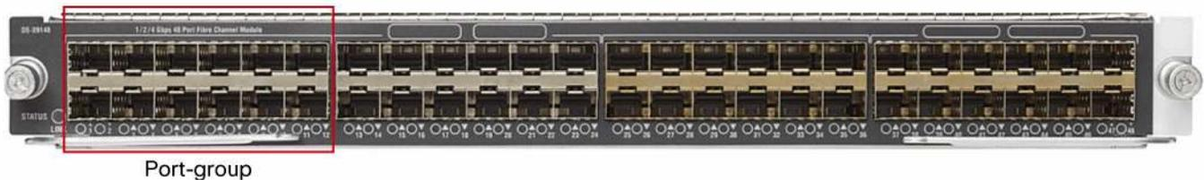
By default, a 12-port linecard offers line-rate throughput at all of 1/2/4 Gbps. The 24-port linecard offers line-rate throughput at 1/2 Gbps but is 2:1 over-subscribed at 4 Gbps if all ports in the same port group are attempting to push line-rate traffic simultaneously. The 48-port linecard offers line-rate throughput at 1 Gbps but is 2:1 and 4:1 over-subscribed respectively for 2 Gbps and 4 Gbps, if all ports in the same port group attempt to push line-rate traffic simultaneously (Table 1).
