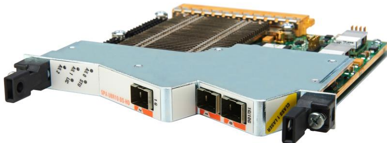
Figure 1. Cisco 3 Gbps Wideband SPA for the Cisco uBR10012 Universal Broadband Router
