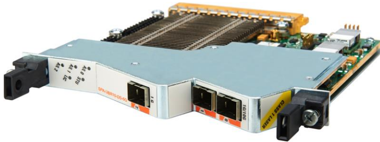
Figure 2. Cisco 6 Gbps Wideband SPA for the Cisco uBR10012 Universal Broadband Router
