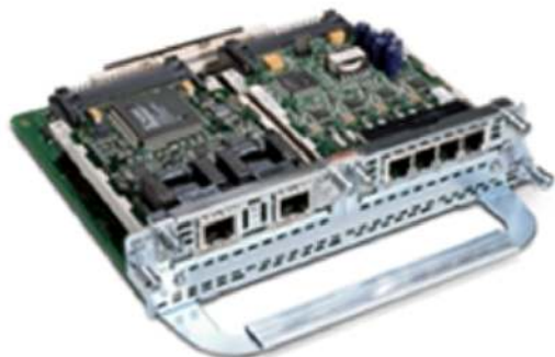
Figure 1. NM-HD-2VE with One VWIC2-2MFT and One VIC3-4FXS/DID
