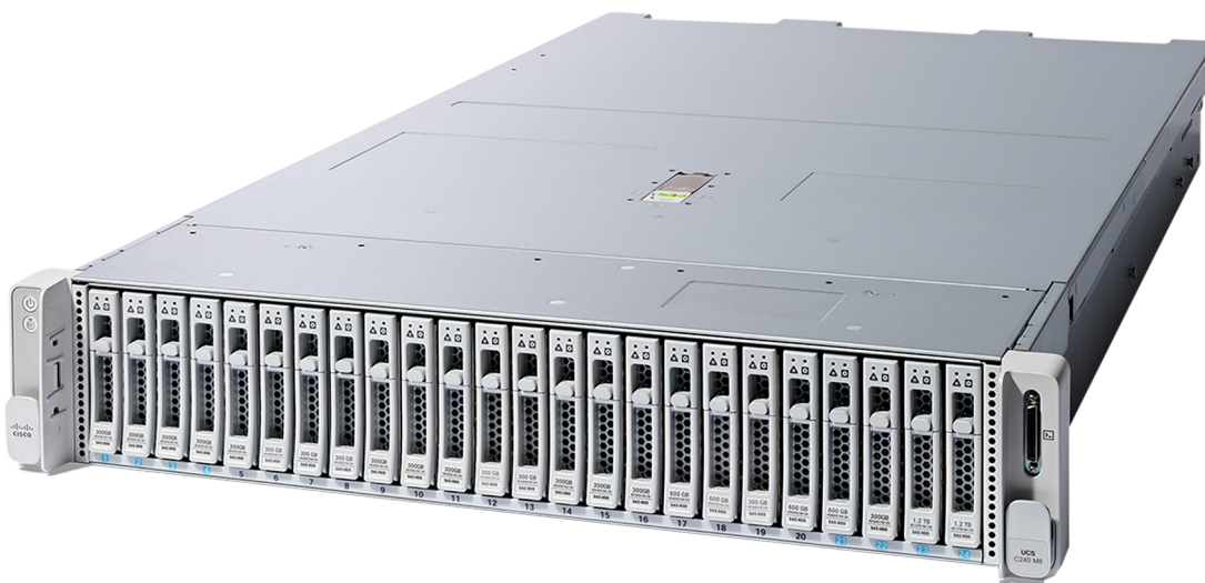
Figure 1. Cisco Compute Hyperconverged with vSAN HCIVS240C M8 All-NVMe Server
