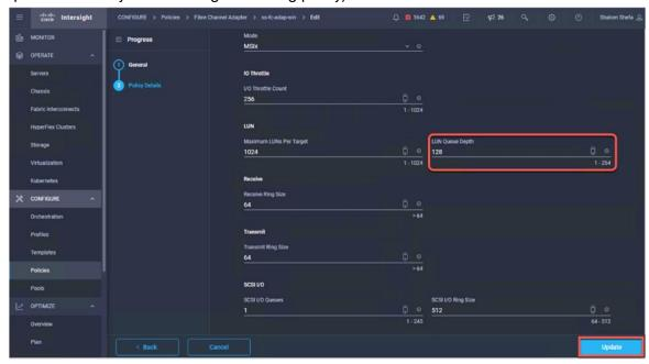
3. Add the Fibre Channel adapter policy to the SAN connectivity policy of the Cisco UCS server profile and deploy or redeploy the server profile.
