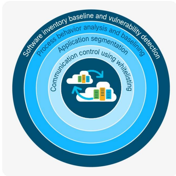
Figure 2. Multidimensional workload protection approach using Cisco Tetration
