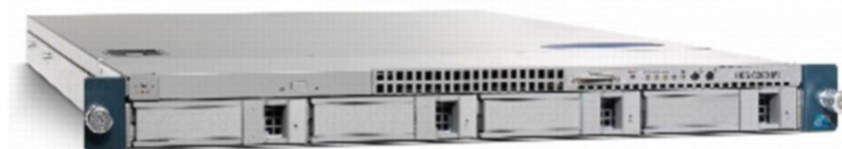
Figure 1. The Cisco UCS C200 M2 High-Density Rack-Mount Server for Cisco DMS Applications
