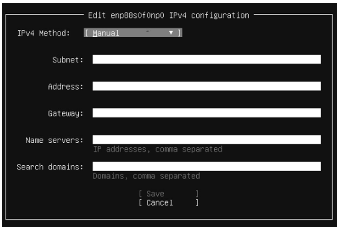
Figure 32. Manual IPv4 configuration for the host management interface
