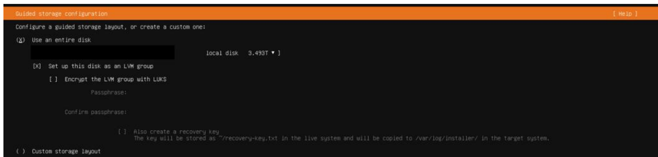
Figure 34. Entire-disk guided storage with LVM selected; the drive identifier is masked
