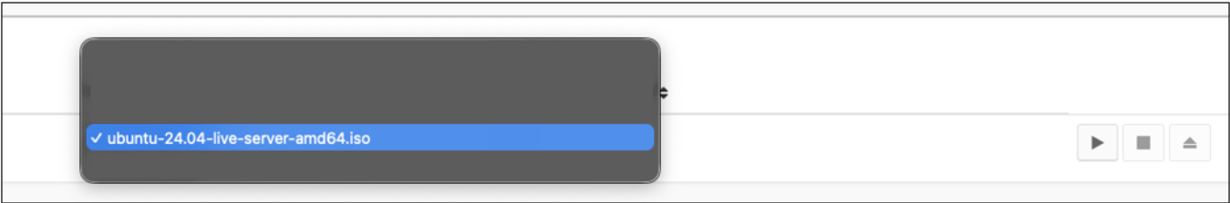
Figure 24. Ubuntu Server ISO selected before starting redirection; unrelated repository entries are masked
