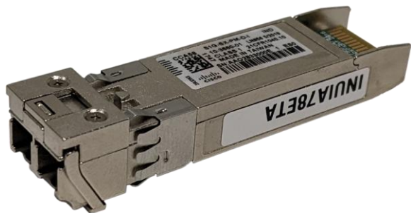
Figure 1. 1G Short-Reach (SX) Transceiver
