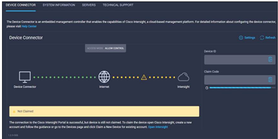
Figure 16. Connect the fabric interconnects to Intersight
