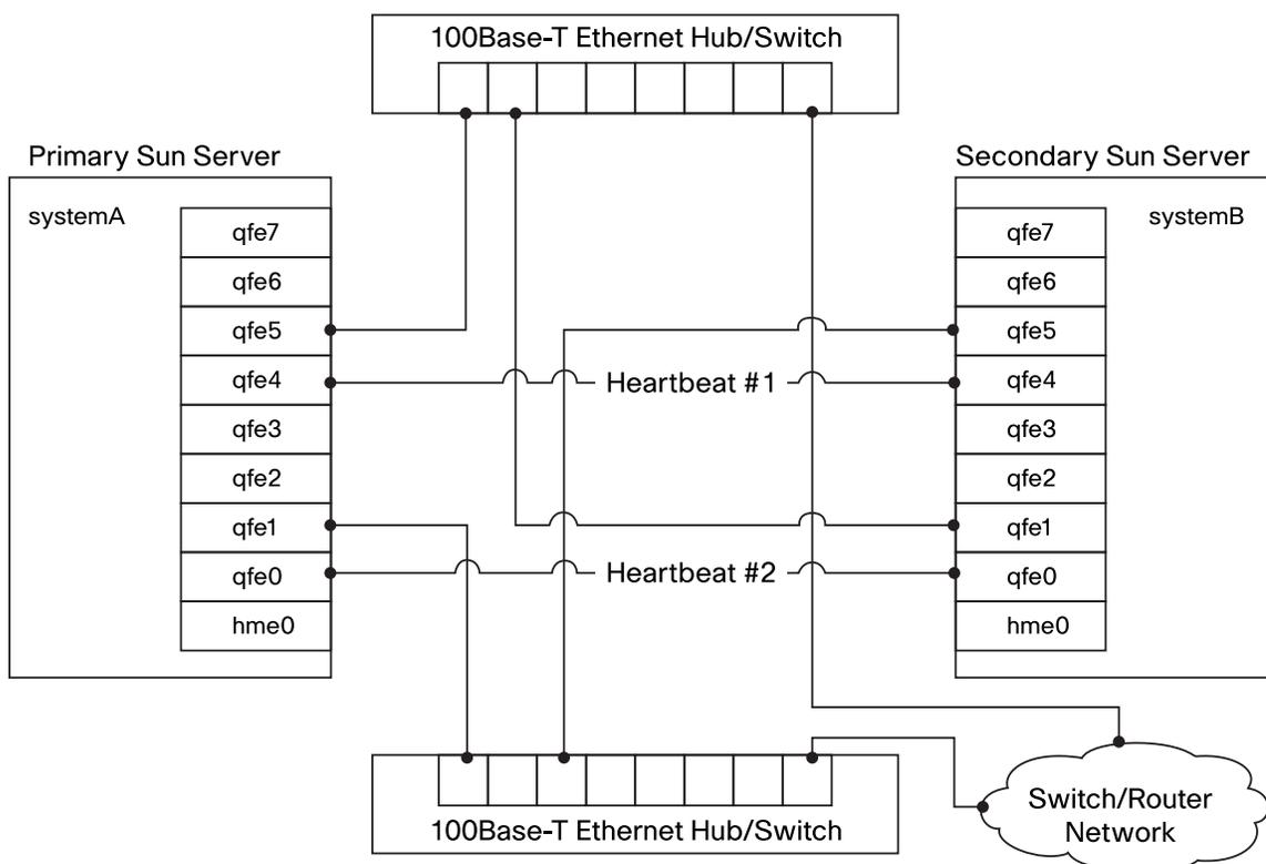
Cluster heartbeat is facilitated using redundant interfaces through direct connect crossover (reversing) Ethernet cables. If the connection between the servers fails, the heartbeat can also be sent across the LAN. Heartbeat messages run across a low latency transport (LLT) protocol, providing the high-speed, low-latency mechanism that Veritas uses for both local and geographical redundancies to help ensure that all nodes get status update information at the same time.
