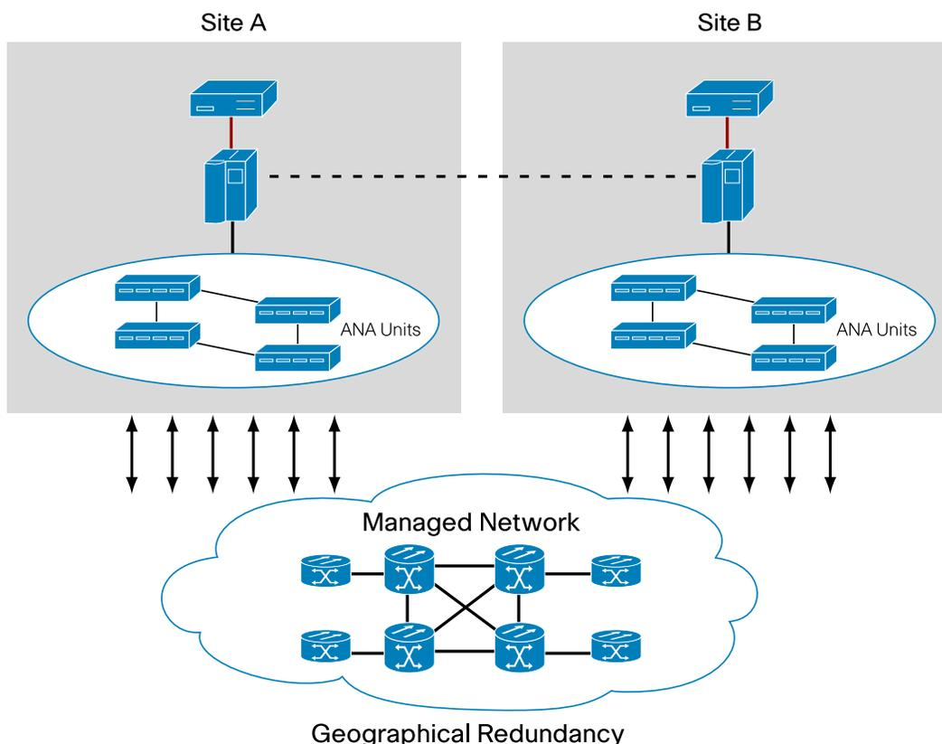
**Split-Brain:** In a geographical redundancy configuration, it is not recommended (even though it is technically possible) to use automatic failover to the standby gateway in order to avoid a "split-brain" scenario where each node in the cluster may mistakenly decide that the other node has gone down and attempt to start services that the other node is still running. This would lead to data corruption in the Oracle database from which it is difficult to recover.
