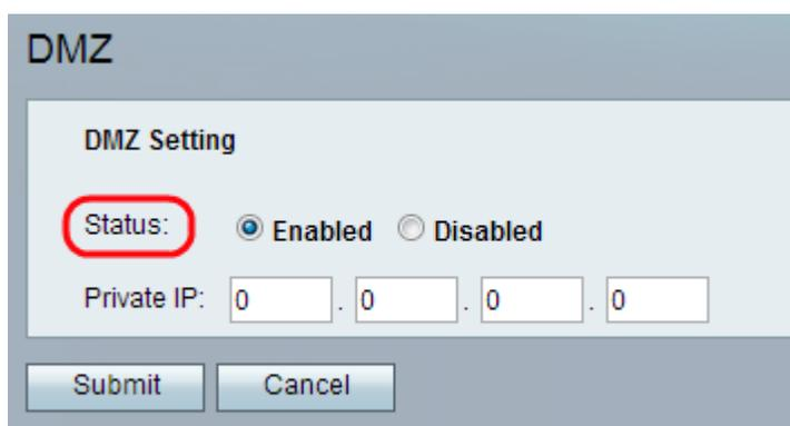
The screenshot shows the 'DMZ' configuration page. Under 'DMZ Setting', the 'Status' is set to 'Enabled' (indicated by a selected radio button, which is circled in red). The 'Private IP' field is set to '0.0.0.0'. There are 'Submit' and 'Cancel' buttons at the bottom.
