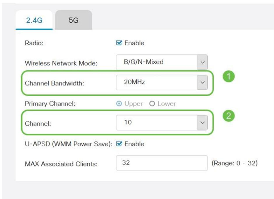
The screenshot shows the wireless settings for the 2.4G band. The 'Radio' is enabled. The 'Wireless Network Mode' is set to 'B/G/N-Mixed'. The 'Channel Bandwidth' dropdown is highlighted with a green box and labeled '1', showing '20MHz'. The 'Primary Channel' is set to 'Upper'. The 'Channel' dropdown is highlighted with a green box and labeled '2', showing '10'. The 'U-APSD (WMM Power Save)' is enabled. The 'MAX Associated Clients' is set to '32' (Range: 0 - 32).
