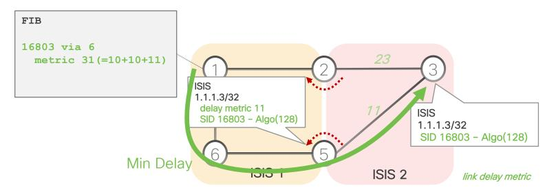
• IGP on Node 1 installs the Algo(128) SID 16803 via the optimal end-to-end min-delay path
