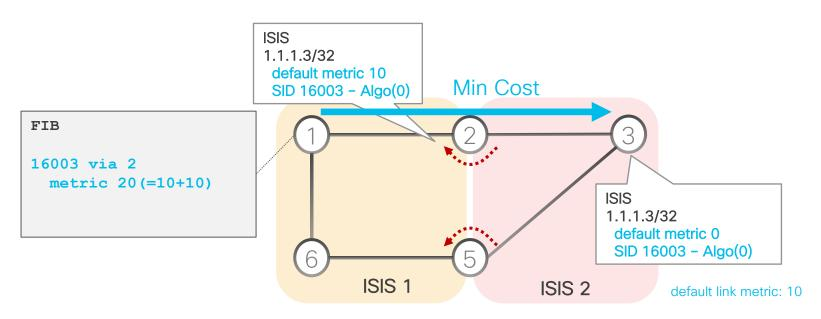
• IGP on Node 1 installs the Algo(0) SID 16003 via the optimal end-to-end min-cost path
