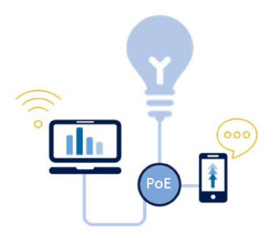
In a connected lighting system that uses Power-over-Ethernet (PoE), each luminaire is directly connected to a building's IT network via an Ethernet cable and PoE switch. Each luminaire has a unique IP address so that it can be individually monitored and managed.
