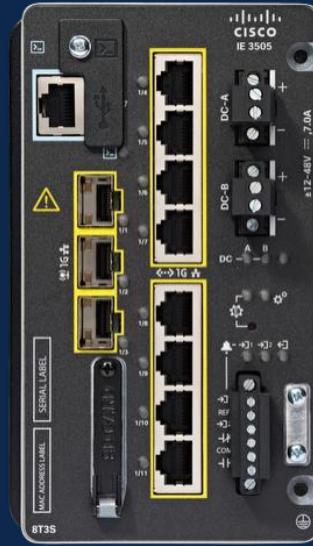
IE-3505-8T3S 8x 1GE ports & 3x 1GE SFP ports HSR/PRP/DLR
