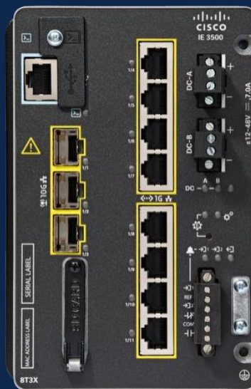
IE-3500-8T3X 8x 1GE ports 3x 10G SFP ports
