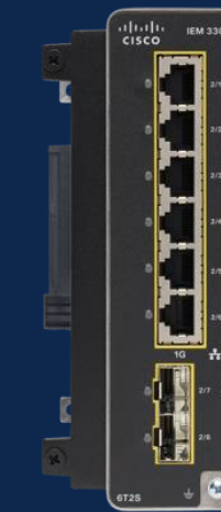
IEM-3500-6T2S 6x 1GE ports 2x 1GE SFP ports
