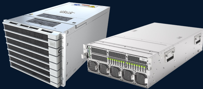
UCS Dense GPU Servers
