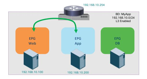
Because this is a communication between two End-points in different EPG, the forwarding decision is made in the leaf switch
