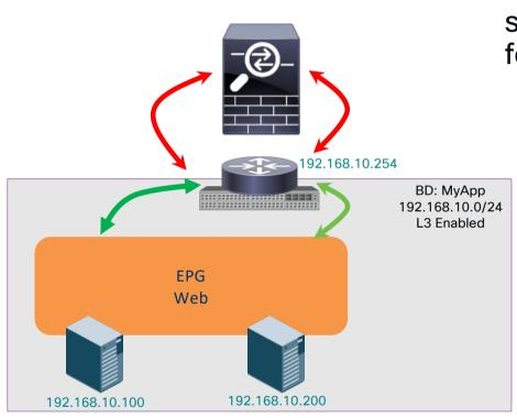
Using PBR, it is possible to attach a service graph to redirect traffic to FTD for traffic inside an EPG
