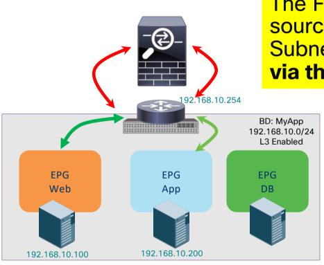
The Firewall must be in **ONE ARM** as source and destination are in the same Subnet. It must **allow traffic in and out via the same interface.**
