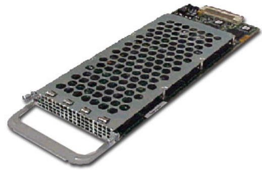
Figure 5 Cisco AS5400 Series 60- and 108-port Feature Card
