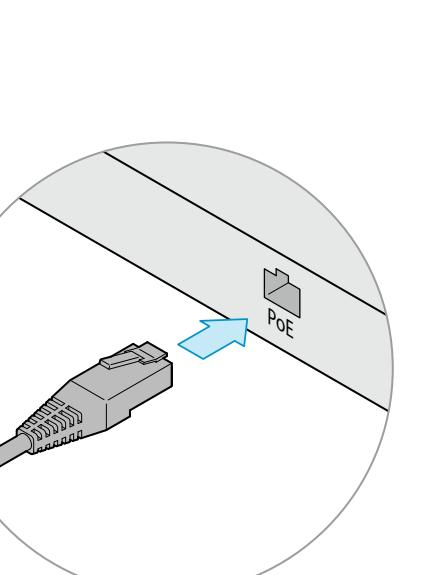
Either connect the microphone to a PoE port on the Cisco collaboration device, or to a PoE port on a switch that is connected to the Cisco collaboration device.
