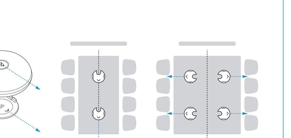
For microphones placed along the table centerline, the arrow should point away from the screen. If not placed along the centerline, the arrow should point toward the sides where people are sitting.
