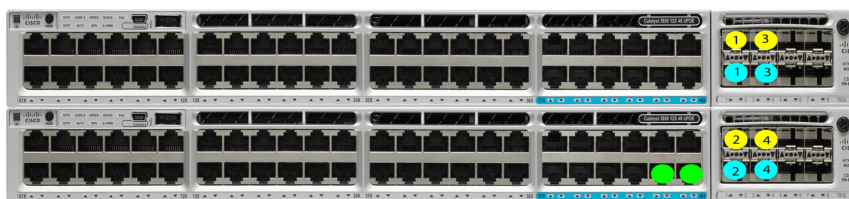
Dual 10/25GE ToR Switches (standalone or stacked)
