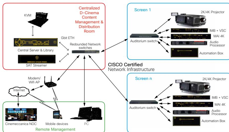
To sustain an High Quality bitstream with a very low latency and delay for the failover procedures, In.I.T srl engineered a Cisco Certified Solution for that IP Network Infrastructure, using, for the Distribution Room, a Stack of Cisco Catalyst 2960S Series Switches, and for the Auditorium Room, the Cisco 300 Series Switches. (For theaters with a large deployment of projectors, the Cisco Catalyst 3750 Series Switches are used)
