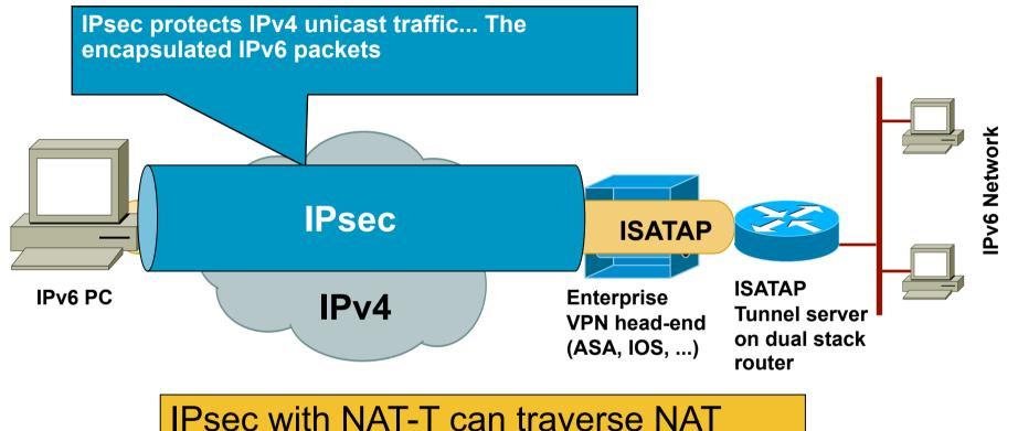
ISATAP encapsulates IPv6 into IPv4
