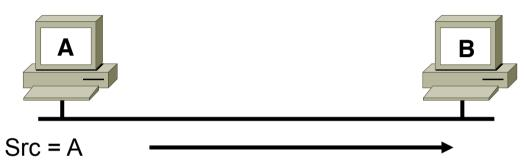
Dst = Solicited-node multicast of B ICMP type = 135 Data = link-layer address of A Query: what is your link address? Security Mechanisms Built into Discovery Protocol = None
