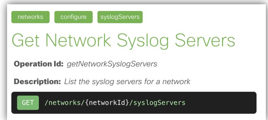
The screenshot shows a developer interface with tabs for networks, configure, and syslogServers. The main content is titled "Get Network Syslog Servers". It includes an "Operation Id: `getNetworkSyslogServers`" and a "Description: List the syslog servers for a network". Below this is a code block for a GET request: `GET /networks/{networkId}/syslogServers`.
