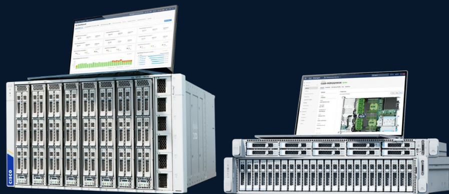
UCS Blade (w/GPU Expansion) and Rack
