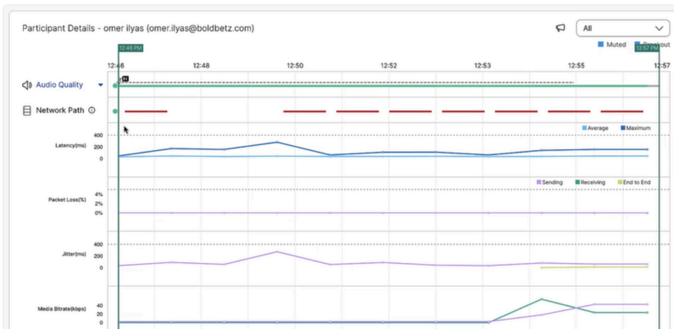
Figure 1.5-2: Network Path after integrating ThousandEyes
