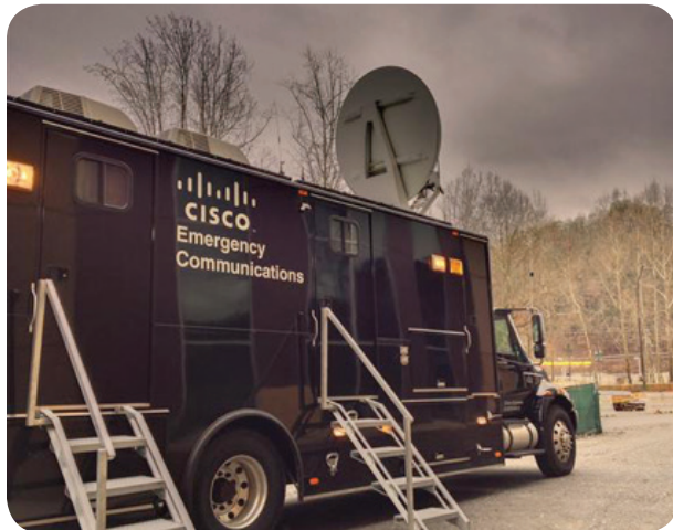
Figure 1: Cisco Network Emergency Response Vehicle
