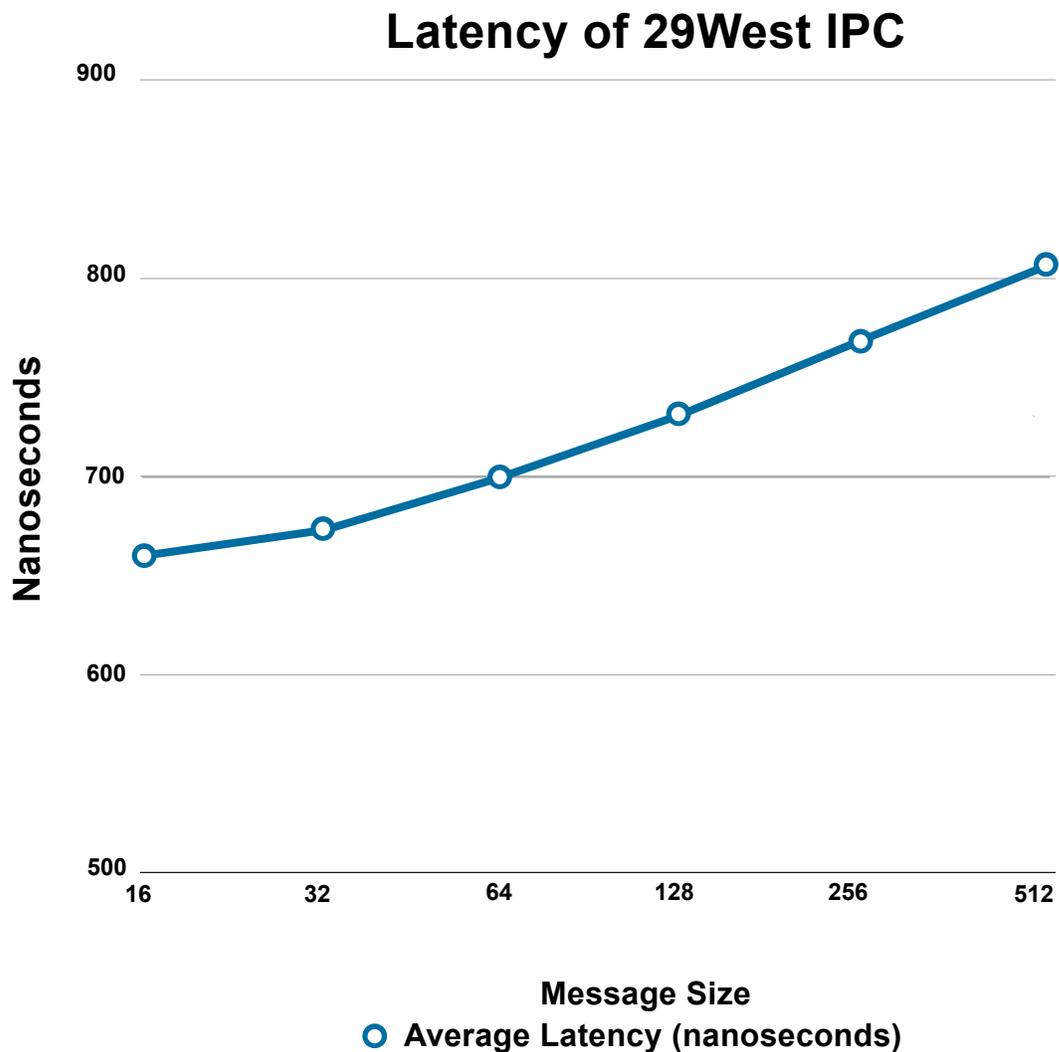
Observed latencies were significantly under 1 microsecond for all message sizes through 512 bytes. This shows an increase in latency as message size increases, similar to all other transports 29West has tested.
