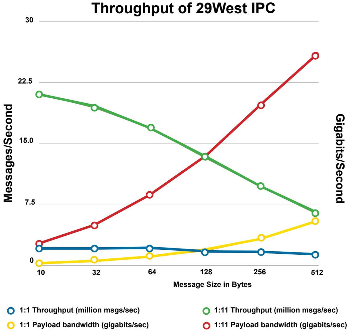
These results show extremely good throughput in both the 1:1 case and the 1:11 fanout case. Over 2 million messages per second per thread is significantly more throughput than any network-based benchmark 29West has ever seen. Not to mention the excellent horizontal scalability shown in the fanout test, which shows a mere 9% drop from perfectly linear scaling.
