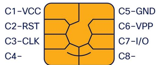
Figure 2: Smartcard pinout diagram
