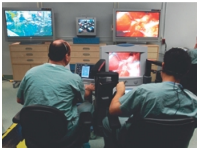
TELEROBOTIC SURGERY: Using real-time video and robotic controls, doctors at St. Joseph's Hospital in Canada perform acid reflux surgery on a patient 400 kilometers away
