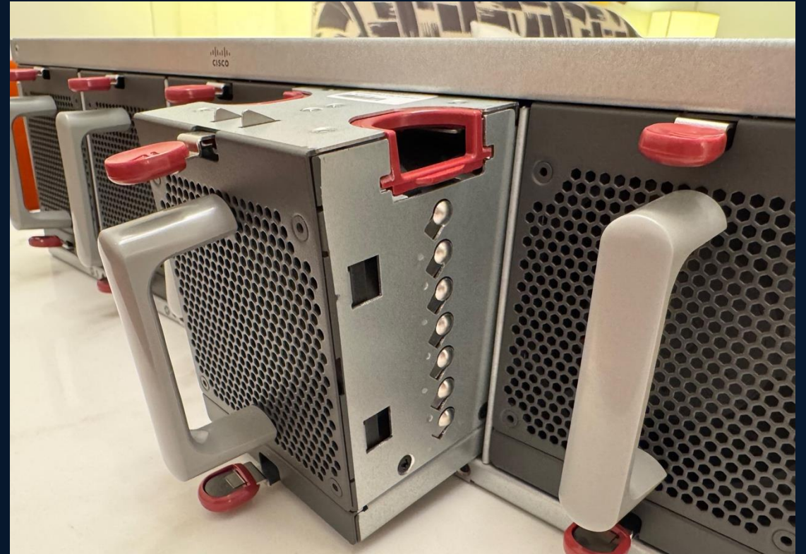
Hot plug fans removed from the back
