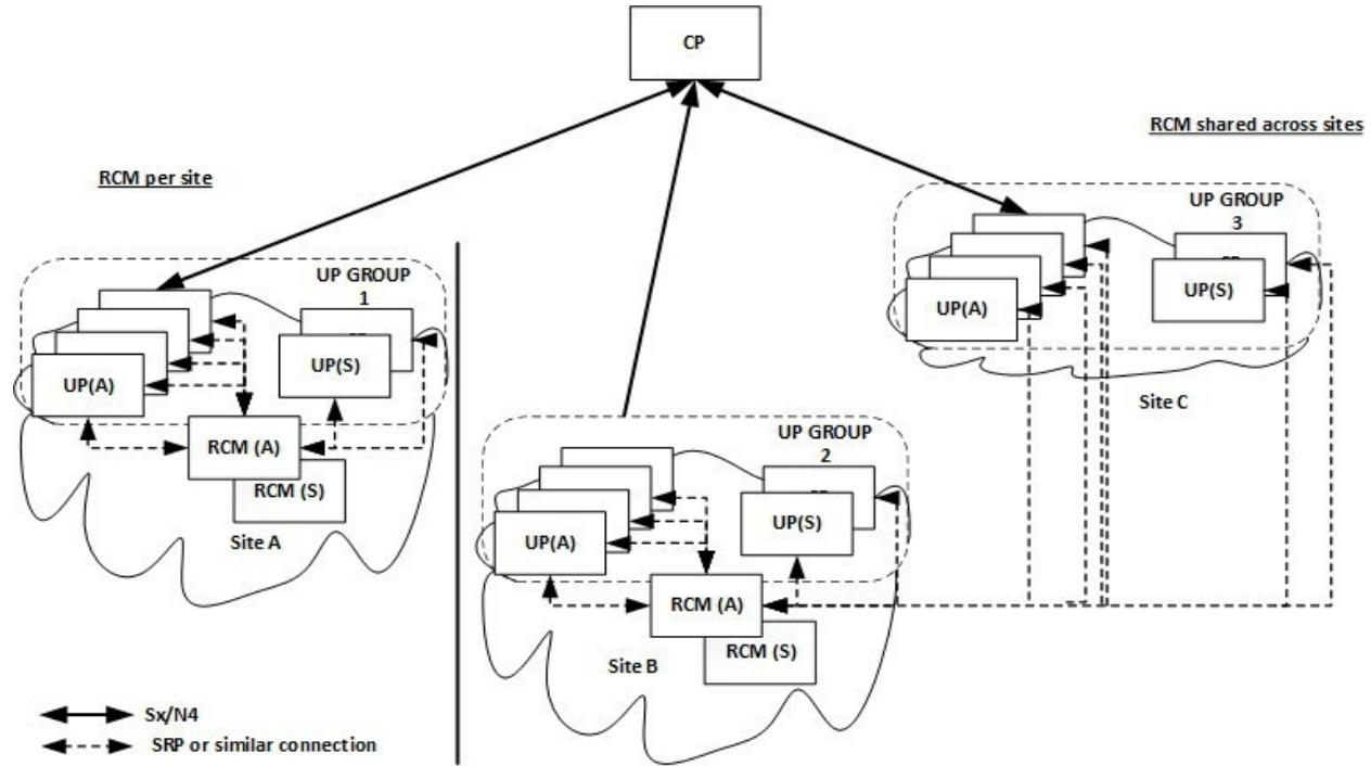
In 4G networks, UPs and CPs communicate over the Sx interface. In 5G, they communicate over N4 interface. The UP is user plane which could be a PGW-U, SGW-U, SAEGW-U, or UP(F). A group of UPs that are deployed to support the same configuration are said to be a part of same UP group (UPG). Therefore, for an N:M redundancy configuration, the UP group is comprised of (N+M) UPs that are of the same capacity and capability.
