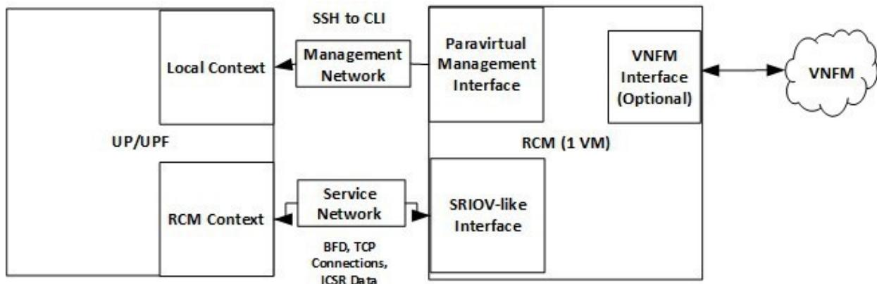
The RCM node is built on Subscriber Management Infrastructure (SMI). SMI provides the Kubernetes (K8s) infrastructure, which is used to bring all the required pods to support the redundancy for UPs.
