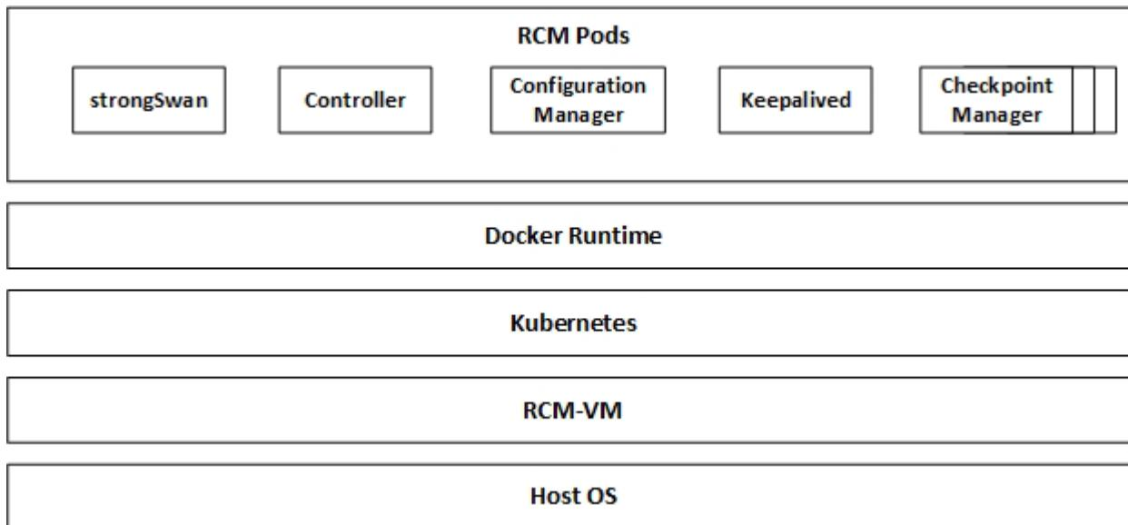
When RCM is deployed on bare metal, the RCM VM layer does not exist, and packet flow involves host kernel.
