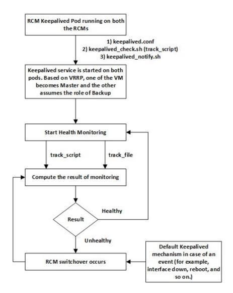
After the Keepalived pod is up and running on both the VMs, one of the RCM VMs comes up as Primary and another as Backup. Keepalived leverages the following files for proper operation:
