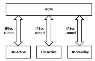
There is one IPSec (L3) tunnel between RCM and each UP. This node-level L3 tunnel between RCM and UP guarantees full protection of information exchanged between RCM and UP.
