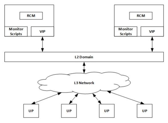
RCM HA deployments require the installation of two RCM instances instead of one. To achieve high-speed communication between the UPs and RCM, and to ensure that the UP switchover time is as minimal as possible, both RCM should be deployed in the same datacenter as the UPs for which they are providing redundancy.
