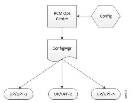
The ConfigMgr Pod is used to take the user input (configuration) from the Ops Center CLI and convert it into the corresponding StarOS CLI. The converted CLI is then pushed to the registered UP/UPF over SSH.
