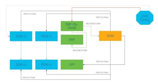
The ConfigMgr Pod is used to take the user input (configuration) from the Ops Center CLI and convert it into the corresponding StarOS CLI. The converted CLI is then pushed to the registered UP/UPF over SSH.
