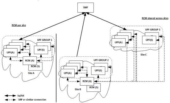
In 4G networks, UPs and CPs communicate over the Sx interface. In 5G, the UPFs and SMFs communicate over N4 interface. The UP is user plane which could be a PGW-U, SGW-U, SAEGW-U, or UP(F). A group of UPs that are deployed to support the same configuration are said to be a part of same UP group (UPG). Therefore, for an N:M redundancy configuration, the UP group is comprised of (N+M) UPs that are of the same capacity and capability.
