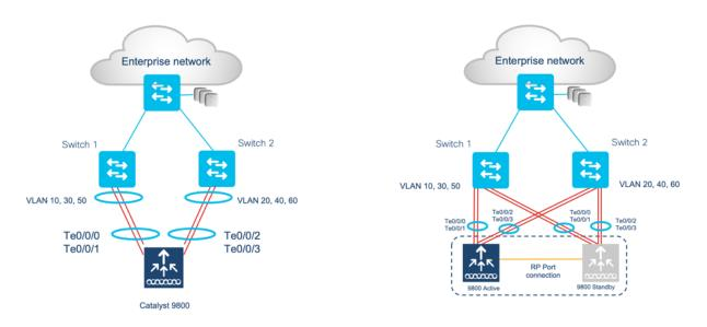
Note: Controller with multiple LAGs can be connected to a single switch, However, different VLANs must be connected to different LAGs
