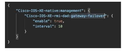
**Configuring Gateway Failure Detection Interval**
