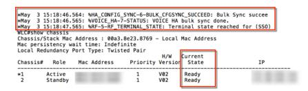
**Note**: Breaking the HA Pair : The HA configuration can be disabled by using the chassis clear command followed by a reload
