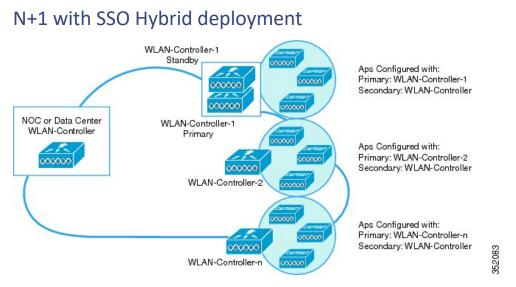
A hybrid topology of SSO redundant pair and N+1 primary, secondary and tertiary model is supported as shown above. The secondary controller at the DR site can be a Catalyst C9800-L, C9800-40 C9800-80 or C9800-CL Wireless controller. Access points failing back from Catalyst 9800 Wireless controller to CUWN controllers will re-download the code before joining the CUWN wireless controller and vice versa.
