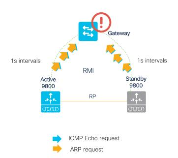
The Catalyst 9800 Wireless controller has two recovery states to prevent an active-active scenario.
