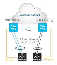
With this topology a single L2 port-channel is created on each box. Enable dot1q to carry multiple VLANs and connect the standby in the same manner. Make sure that switch can scale in terms of ARP and MAC table entries.
