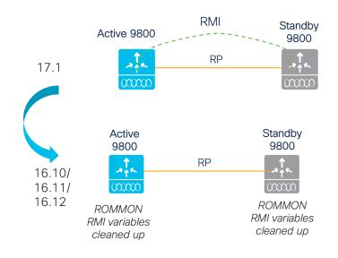
If RP based configuration was used, after downgrade the system will continue to use RP-based configuration
