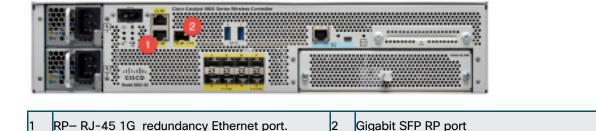
Both C9800-40-K9 and C9800-80-K9 Wireless controllers have two RP Ports as shown in the figures
