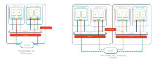
The figure on the left shows Redundant port connected on the same server.
