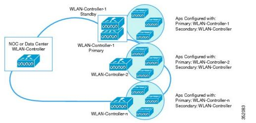
A hybrid topology of SSO redundant pair and N+1 primary, secondary and tertiary model is supported as shown above. The secondary controller at the DR site can be a Catalyst C9800-L, C9800-40 C9800-80 or C9800-CL Wireless controller. Access points failing back from Catalyst 9800 Wireless controller to CUWN controllers will re-download the code before joining the CUWN wireless controller and vice versa.
