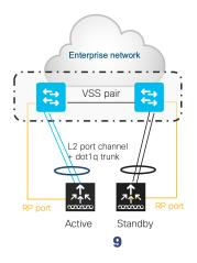
Connecting a C9800 wireless controller HA pair to upstream switches with Release 17.1 and above
