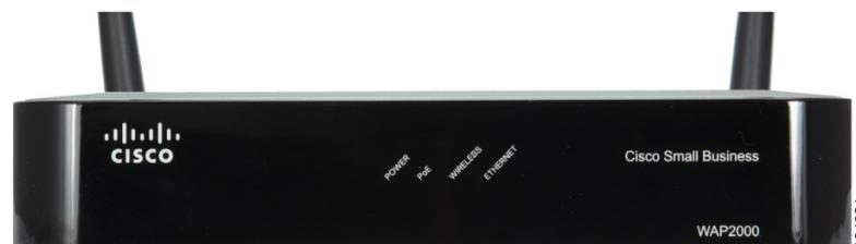
**POWER**—(Green) Lights up when the access point is powered on.
