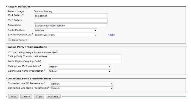
When nnnn@exp.domain is dialed by an endpoint registered to Unified CM, Unified CM will route the call to the Expressway as nnnn@<FQDN of Expressway>:5060 (TCP) or nnnn@<FQDN of Expressway>:5061 (TLS). (The domain may alternatively be the IP address of Expressway, depending on what is configured as the SIP Trunk **Destination Address**.)
