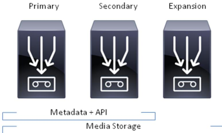
All servers are deployed on the same hardware and virtual machine, and all are provided with the same installed software. They differ only in function. The Primary server is always the first server to be installed, and is identified as such during the installation process. Secondary and Expansion servers are identified during the initial configuration process, after installation has completed.
