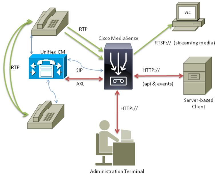
Though this diagram shows only one Cisco MediaSense server and one Unified CM server, each should be considered as a cluster of such servers. That is, one cluster of Cisco MediaSense servers interacts with one cluster of Unified CM servers. From a Unified CM perspective, there is no concept of a hierarchy of recording servers. SIP Trunks should be configured to point to all Cisco MediaSense servers.
