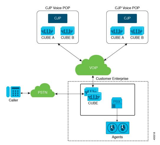
In some cases, the customer enterprise owns and operates the CUBE and the PBX, which eliminates the need for a SIP header.
