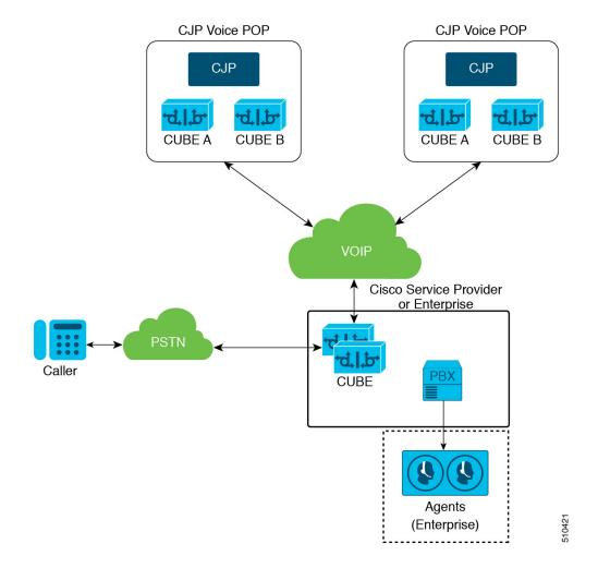
Either the service provider or the customer enterprise can own and operate the CUBE and the PBX. In this case:
