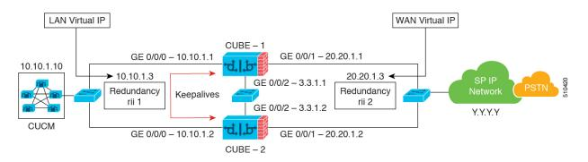
Using the CUBE High Availability (HA) feature with box-to-box redundancy ensures that the system preserves active calls when one of the CUBEs experiences an outage. Using the CUBE HA feature requires that all CUBEs:
