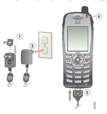
AC plug adapter—Insert the AC plug adapter into the slot on the power supply.
