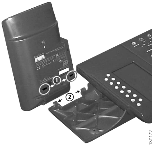
Figure 4 Connecting the Expansion Module
